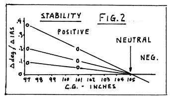
Hopefully the point of neutral stability will be aft of your c.g. range, as it is in our airplane. You should not fly your airplane at a c.g. where the stability is negative, so if the point of neutral stability turns out to be forward of 102.0, you must either restrict your aft c.g. range, or increase the incidence of your canard. That is the bottom line.
