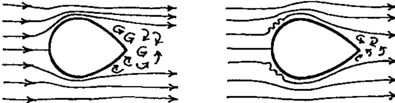
Laminar BL allows more pressure drag than Turbulent BL
