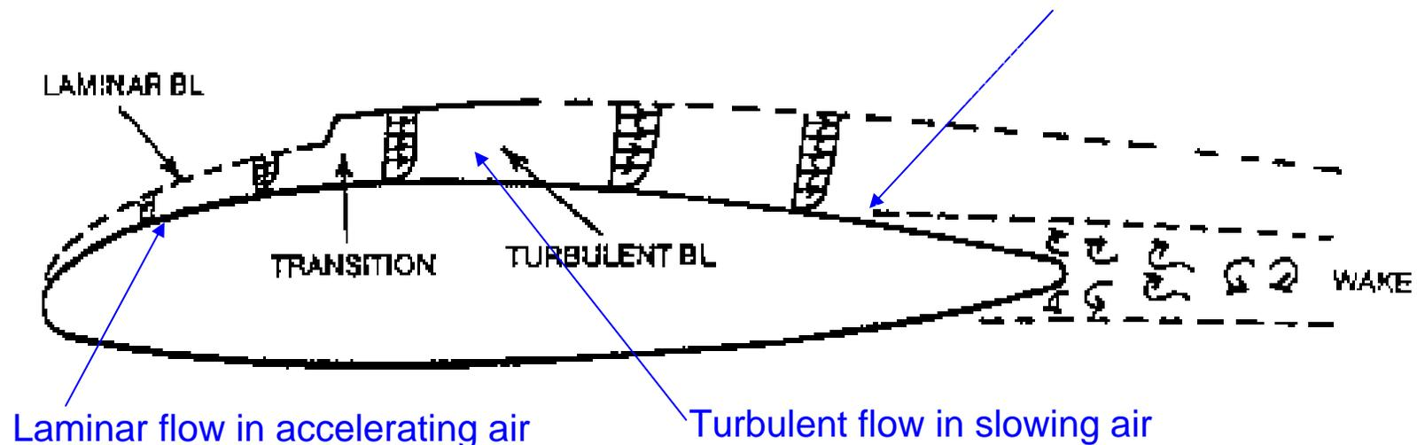
**Fig. 5.24** An enlarged view of the boundary layer above a lifting airfoil
