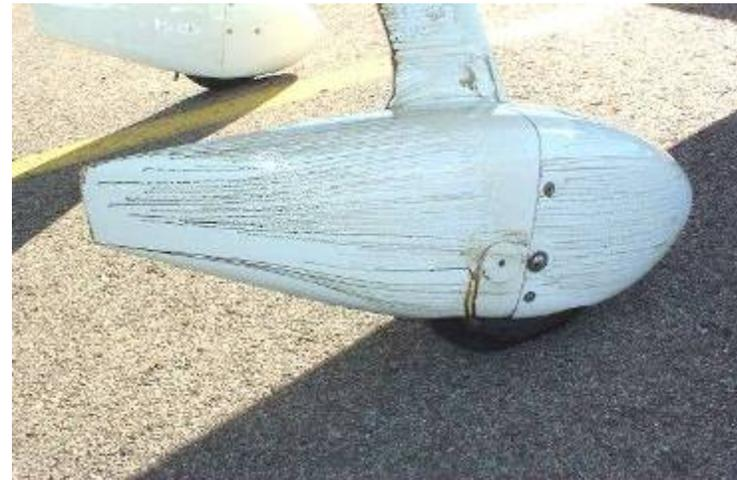
\*Hoerner specifies 3.7 to 1 t/c or 27% thick for an optimum trade between profile and skin friction drag
